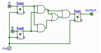
The maximum allowable hold time for RegC is how long it takes for RegC's input to change, so (clk-to-q of A or B) + shortest CL time = 4 + (5 + 5) = 14 ns.
