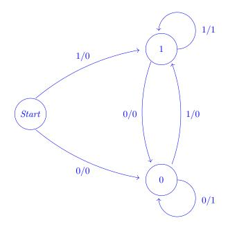
6.3 Draw an FSM that will output a 1 if it recognizes the regex pattern {10+1}. (That is, if the input forms a pattern of a 1, followed by one or more 0s, followed by a 1.)
