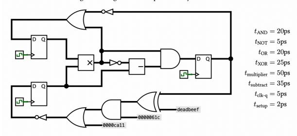
Q6.4 (2 points) Suppose this circuit only deals with two's complement integers. Currently, the subtractor component has a delay of 35ps. What is the maximum delay an adder component can have such that we could replace the subtractor component with adders, NOT gates, and constants to achieve the same delay as the subtractor while maintaining the same behavior? You may assume that constants have no delay.
