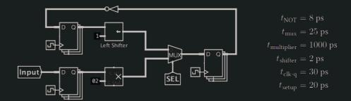
The left shifter combinational logic block shifts the top input by the number of bits indicated by the bottom input. The shifter in the diagram shifts the output of the connected register left by 1 bit.
