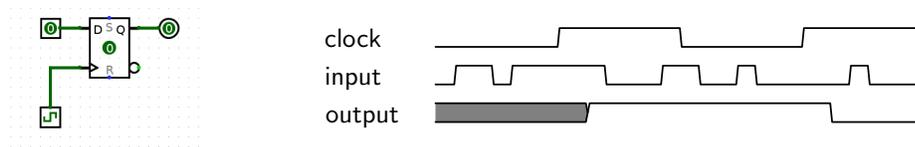
You’ll notice that the value of the output in the diagram above doesn’t change immediately after the rising edge of the clock. Until enough time has passed for the output to reflect the input, the value held by the output is garbage; this is represented by the shaded gray part of the output graph. Clock cycle time must be small enough that inputs to registers don’t change within the hold time and large enough to account for clk-to-q times, setup times, and combinational logic delays.
