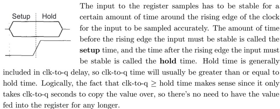
For the following register circuit, assume **setup** of 2.5ps, **hold** time of 1.5ps, and a **clk-to-q** time of 1.5ps. The clock signal has a period of 13ps.
