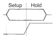
The input to the register samples has to be stable for a certain amount of time around the rising edge of the clock for the input to be sampled accurately. The amount of time before the rising edge the input must be stable is called the **setup** time, and the time after the rising edge the input must be stable is called the **hold** time. Hold time is generally included in clk-to-q delay, so clk-to-q time will usually be greater than or equal to hold time.
