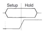
The input to the register samples has to be stable for a certain amount of time around the rising edge of the clock for the input to be sampled accurately. The amount of time before the rising edge the input must be stable is called the **setup** time, and the time after the rising edge the input must be stable is called the **hold** time. Hold time is generally included in clk-toq delay, so clk-to-q time will usually be greater than or equal to hold time.
