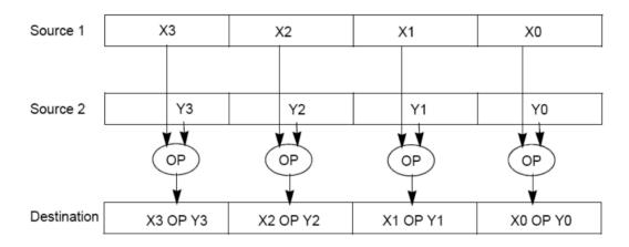
Some machines with x86 architectures can use Intel Intrinsics (Intel proprietary technology) which allow us to use these wider "vector" registers to harness the power of DLP in C code.
