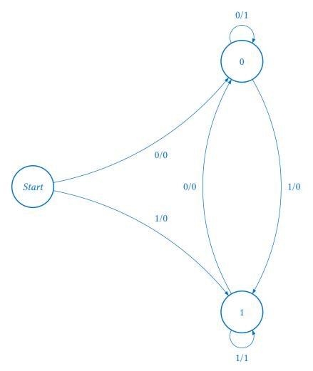
5.3 Draw an FSM that will output a 1 if it recognizes the regex pattern {10+1}. That is, if the input forms a pattern of a 1, followed by one or more 0s, followed by a 1.
