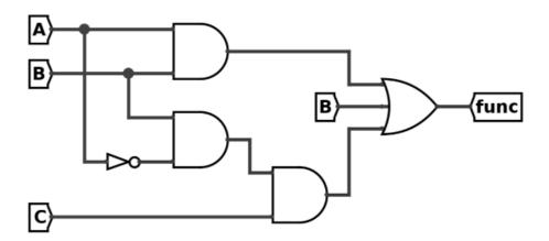
We can label the outputs of each gate in the circuit. In the first layer, we two AND gates for AB and  $\overline{A}B$ . The final AND gate takes  $\overline{A}B$  as its first input and C as its second input for a combined output of  $\overline{A}BC$ . Lastly, an OR gate combines the previous gates with the input B for the final function of  $F(A, B, C) = AB + \overline{A}BC + B$
