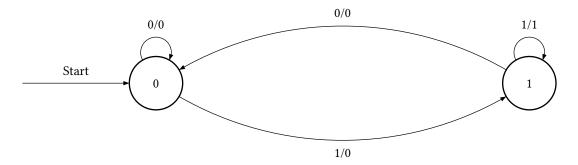
The FSM outputs a 1 if it detects the pattern 11. The FSM would output 001000000110.
